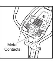
metal contacts. Avoid moving your hands or squeezing the handgrips too tightly; excessive movement or pressure may interfere with heart rate readings. When your pulse is detected, the heart-shaped indicator in the large display will flash each time your heart beats, and your heart rate will be shown.
